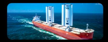
Mitsubishi's *Pyxis Ocean* set sail on its maiden voyage powered by WindWings, an advanced wind propulsion system. The *Pyxis Ocean* is retrofitted with two 37.5m-tall sails, with each wing saving 1.5 tons of fuel, or 4.65 tons of CO₂ emissions, per day.
